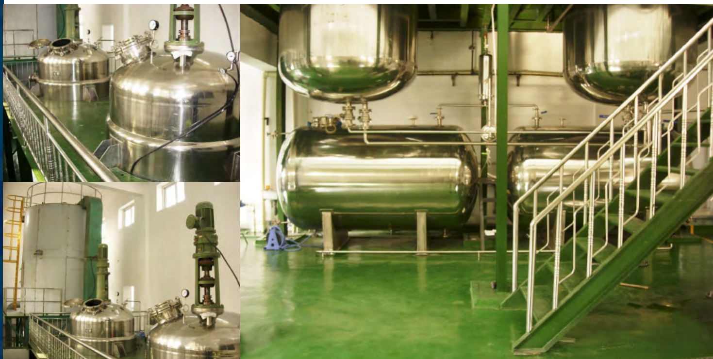
Figure 1. Thousand tons/year oligosaccharide enzymatic process production device
