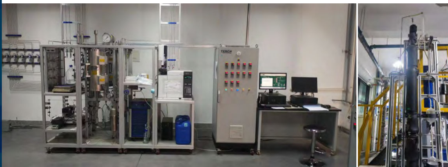
Figure 2. Fixed-bed reaction system as well as product purification system
