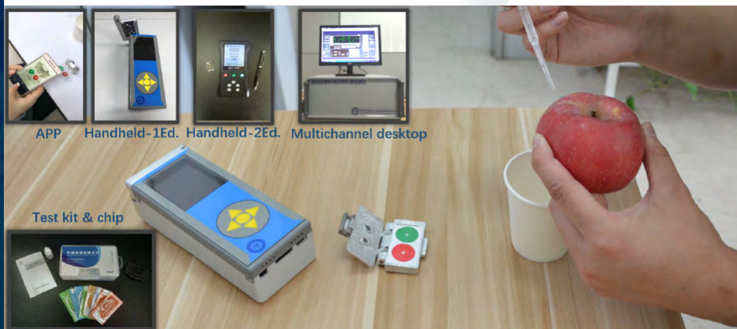
Figure1: Rapid test strips and detectors based on multiple pesticides rapid detection technology
